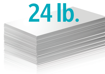
A ream of 500 sheets of 17" x 22" Bond paper that weighs 24 pounds. The thicker paper results in a taller, heavier ream.
